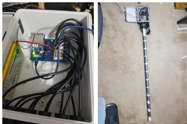
First PCB assembled with modem in weatherproof box (L); station wired and attached to the PVC pole with tape (R). Photos by the author.
