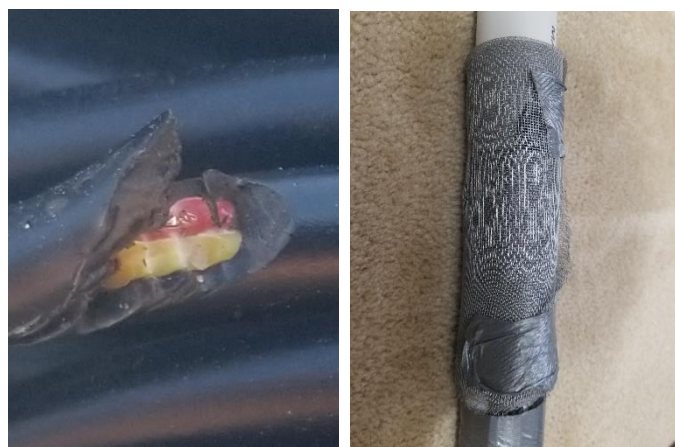
Wire damage caused by mice (L); aluminum window screen used to protect wires from mice (R). Photos by the author.
